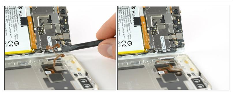
Disconnect the fingerprint sensor using a spudger.
