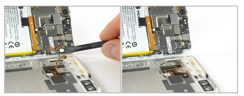
Disconnect the fingerprint sensor using a spudger.
