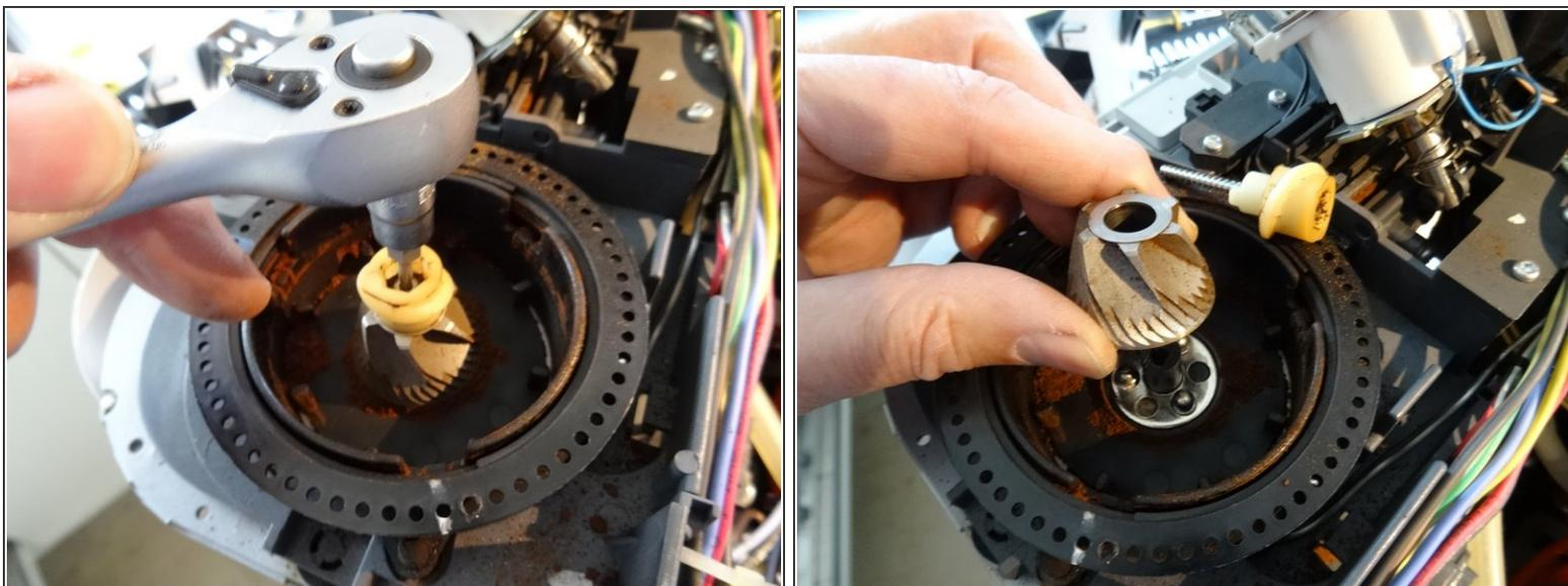
**⚠** The Phillips screw, which holds the milling cone has a left-hand thread, so "wrong turn" turn! The screw is often hidden under parts of coffee beans.
