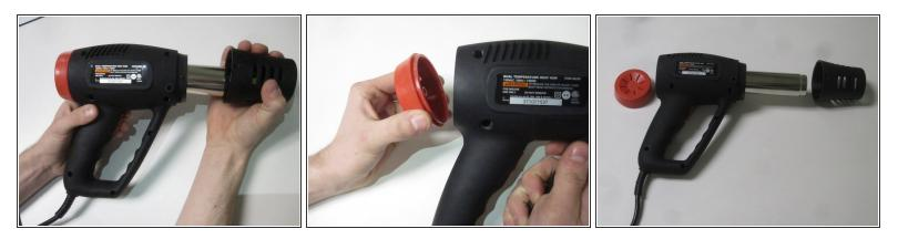
• Remove the barrel casing on either end by twisting and pulling each side off.
