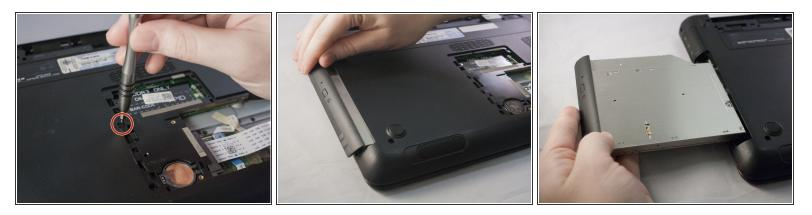
• Unscrew one 3.85mm screw using the PH0 tip and remove from the disk drive.
