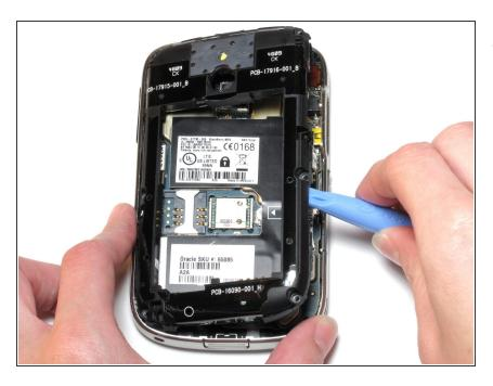
Use the plastic opening tool to remove the rear case.
