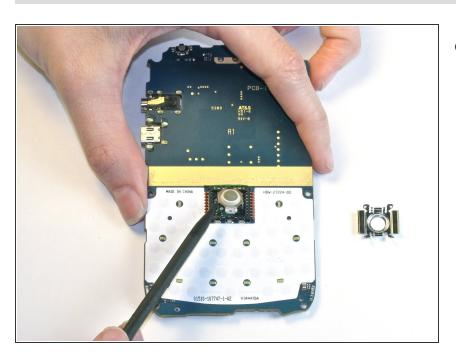
Lift the trackball out of its socket.
