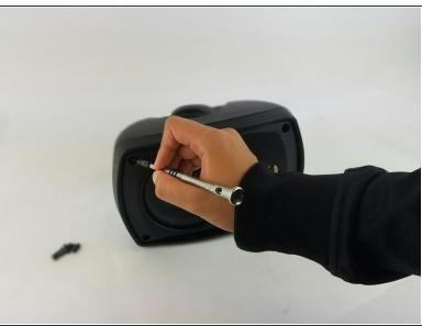
Remove the six Phillips Head 1.2mm screws on the front side of the speaker.
