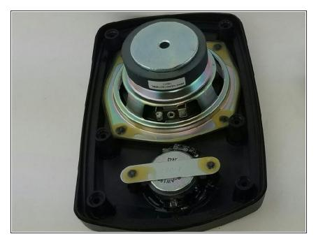
Once the wire assembly is removed, the entire front panel and speaker housing should be separated to replace.
