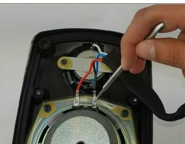
Use the metal spudger to bend down the metal tabs that hold the wires to the terminals. The tabs are small and in between the grooves of the terminal.
