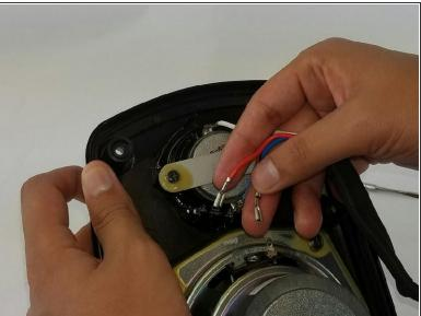
Remove the wires from the terminals.
