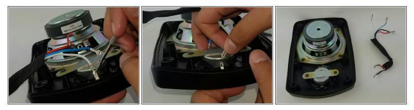
Remove the wires from the terminals. Then remove the entire wire assembly.
