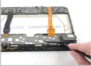
Use the pointed end of a spudger to pry upwards between the other speaker unit and the display chassis. To reassemble your device, follow these instructions in reverse order.
