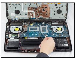
• Unplug the two sets of wires from the motherboard.
