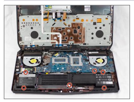
Remove the six 4mm Phillips #1 screws holding the battery in place.
