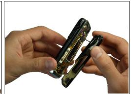
**Caution:** Wires and ribbon connect the front case to the main body. Exhibit care when separating front case from the main body as to not break the connections.
