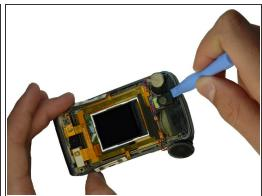
**Caution:** The wiring on the ribbon connector is delicate. Do not excessively pull on the wires.
