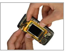
Use the spudger to unclip the two upper wiring connections.
