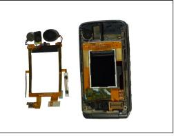
Caution: The ribbon contains important wiring and is glued to the phone. Be careful when removing the ribbon.
