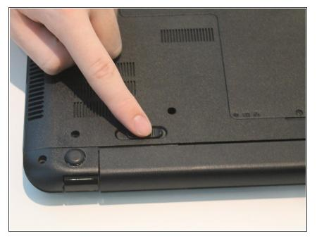
Move the left switch to the right, covering the battery symbol, and hold.
