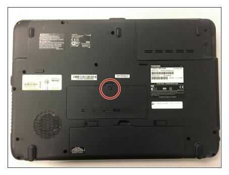
Unscrew 1 Phillips #0 7-mm screw on the back of the computer.
