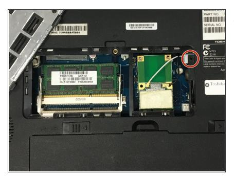
Unscrew the 1 Phillips #0 7-mm screw, located on the right side where the silver tabs of the optical drive poke out.
