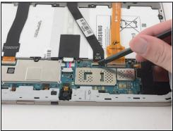
• Use the flat end of a nlyon spudger to pry up the **black** plastic tabs securing the two ZIF connectors.
