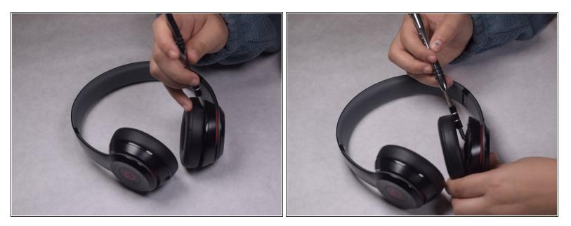
Remove the ear cushions from the headset. The preferred method to do this is to use a screwdriver and pry the cushions off.
