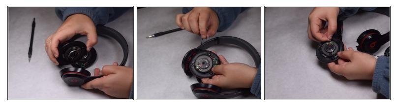
• After you have removed the second internal speaker, you can begin the process of removing the wire. BE CAREFUL with this step, make sure you don't pull off the circuit board.
