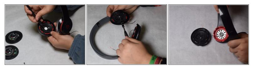
• Now we are going to remove the circuit board holder. Take off the white cover to get access to the screw. Then remove the screw and circuit board holder.
