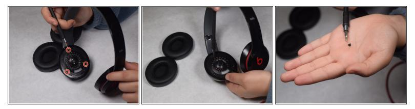
• Remove the screws from both ear bases.
