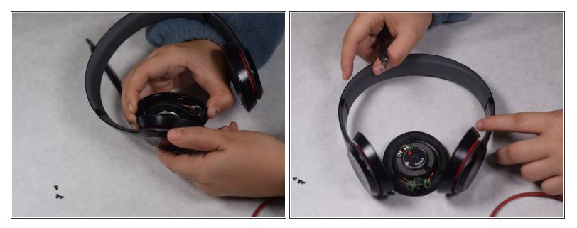
• Once the screws are removed, pop off the inner speakers. Do this for both sides
