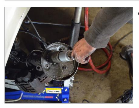
Grab the top of the strut and pull it out of the strut assembly.
