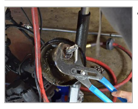
Use a large adjustable wrench or pair of groove joint pliers to remove the strut gland nut.
