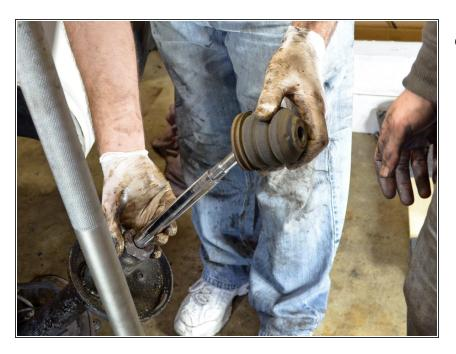
Remove the rubber bump stop from the strut assembly.
