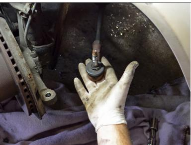
Place a tie rod end puller over the exposed threads of the tie rod end and turn the puller with a socket wrench to push the tie rod end out of the steering knuckle.
