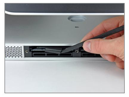
• Use your fingers or the tip of a spudger to slide the black plastic RAM tray pull tab out of the RAM slot.
