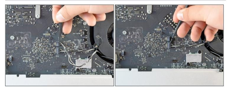
• Release the right and left speaker connectors from their sockets using the flat end of a spudger.
