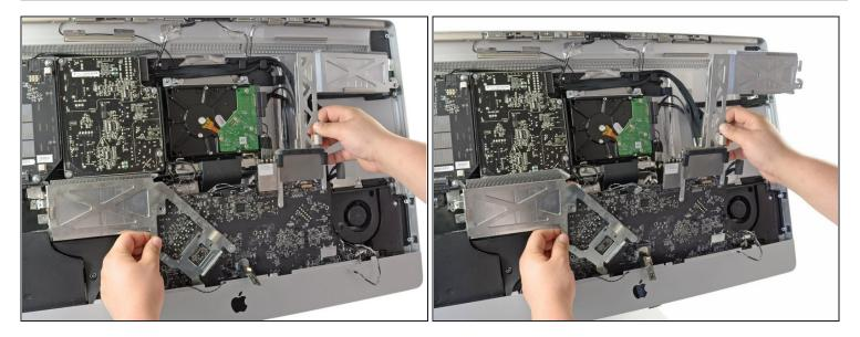
• Simultaneously lift and rotate the logic board and heat sink assembly away from the iMac case until you can easily access the back side of the logic board.
