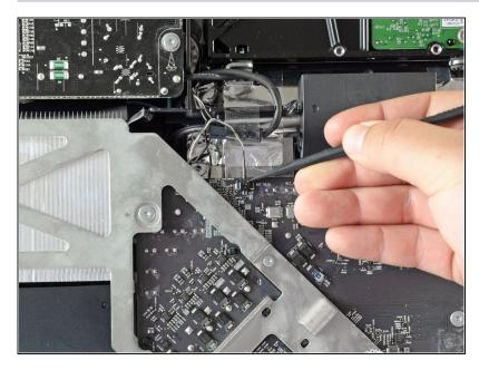
• Push the thermal sensor connector out of its socket with the flat end of a spudger.
