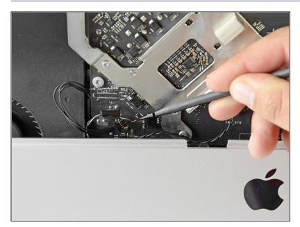
• Use the flat end of the spudger to push the ambient temperature sensor connector out of its socket.
