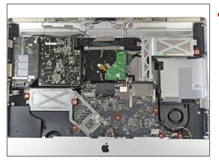
Remove the eight T10 Torx screws securing the logic board and heat sink assembly to the iMac case.
