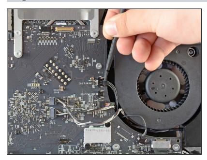
• Use the flat end of a spudger to pull the optical drive fan connector out of its socket.
