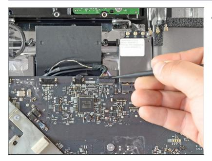
Use the flat edge of a spudger to push the camera/Bluetooth/ambient light sensor connector out of its socket.
