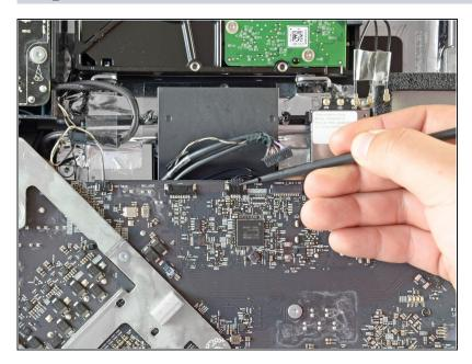
• Release the hard drive fan connector from its socket by pushing on its tabs using the flat end of a spudger.
