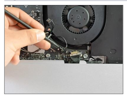
• Use the flat end of the spudger to pull the microphone cable connector free of its socket.
