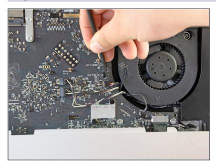
• Use the tip of a spudger to pull the SD board data cable connector out of its socket.
