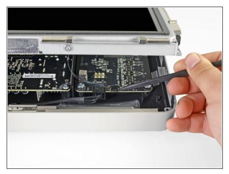
Disconnect the vertical sync cable in the upper left corner of the screen.
