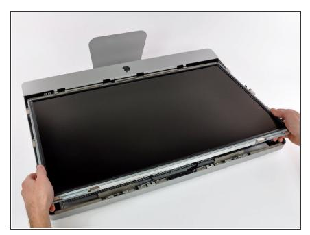
Carefully pull the display toward the top edge of your iMac and lift it out of the iMac case.
