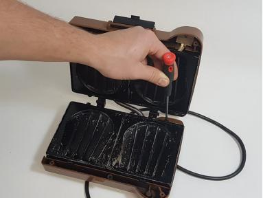
Remove the two screws at the back of the heating plate as shown in the pictures.
