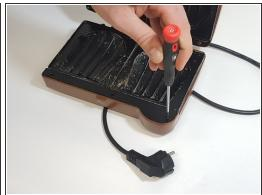
Remove the screws of the front plate, by using a Philips #1 Screwdriver
