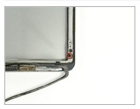
Remove the 2.2 mm Phillips screw located near the bottom right corner securing the AirPort/iSight cable to the display assembly
