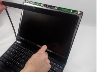
Pull the plastic covering of the screen towards the keyboard, exposing the inner workings of the screen.
