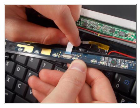
Flip the Power/Audio bar over exposing the ribbon wire and its connection to the Power/Audio bar.
