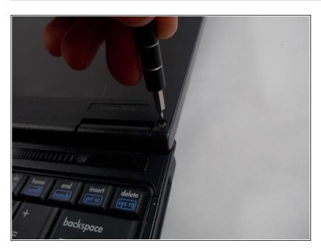
Once the rubber has been removed a screw will be revealed. Remove each of the four screws with your Philips head screwdriver.
