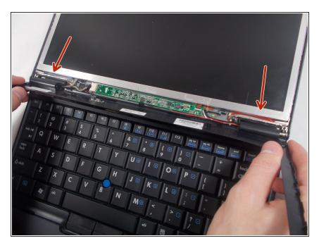
Locate the hinges at the bottom left, and right of the screen
