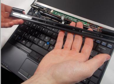
Separate the Power/Audio bar from the hinge by gently pulling.
