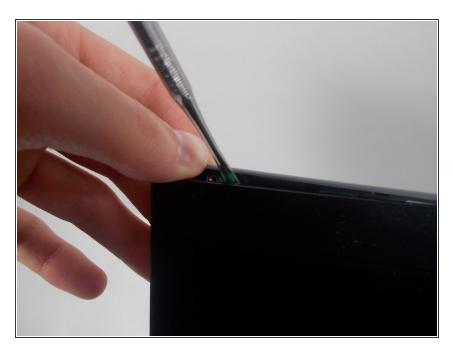
Insert your spudger along the top of the screen, separating the plastic cover and the screen
