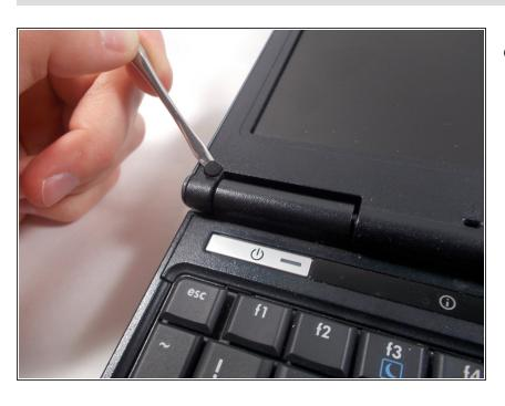
Use a Flathead screwdriver to remove the 4 rubber covers over the 4 screws referenced in step 1.
