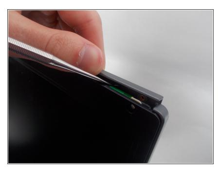
Continue running your Flathead along the top of the screen until the top is completely separated.
