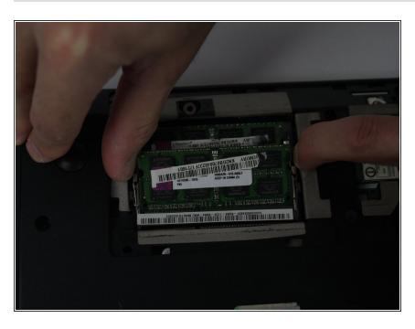
On both sides of the ram, gently grip the sides and pull out of the slot
