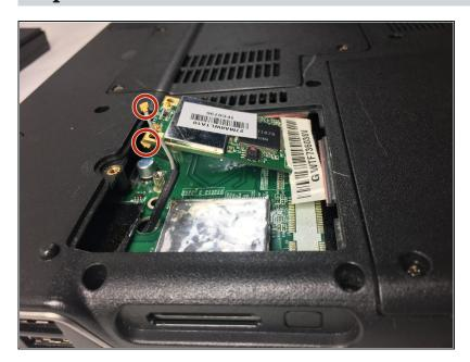
Remove the two wires connected to the wireless card.
