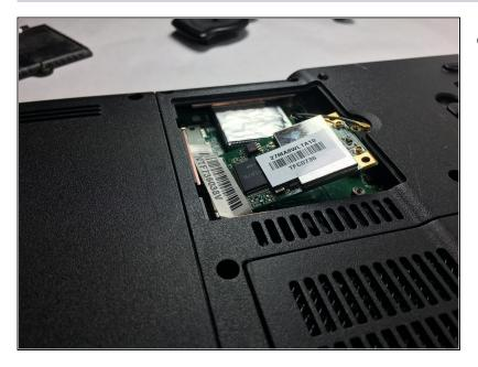
Pull the wireless card's cover plate up and off to reveal the card as shown.
