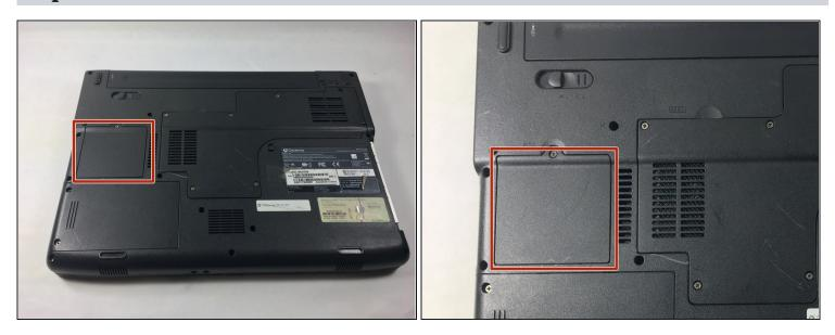
• Locate the wireless card cover, found on the middle-left section of the laptop as shown.
