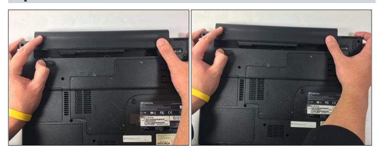
• With both latches unlocked you can now slide out the battery, by pushing it off the top.
