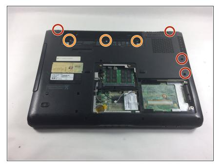
Remove all 4 of the 7.0mm screws and the 3 silver, smaller 4.0mm screws inside the cavity of the battery
