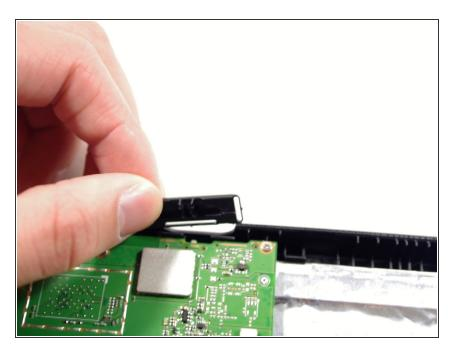
The button can be easily removed and can now be replaced
