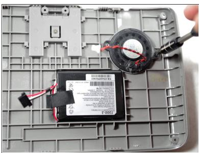
Unscrew the left and the right screws using the ifixit screwdriver.
