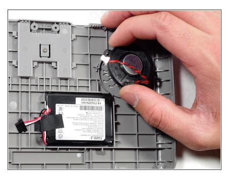
Now that you removed the screws, you can finally replace the speaker.
