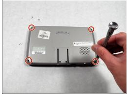
Unscrew four Phillips #0 screws from the back panel.
