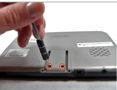
Unscrew two Phillips #0 screws from the back panel.
