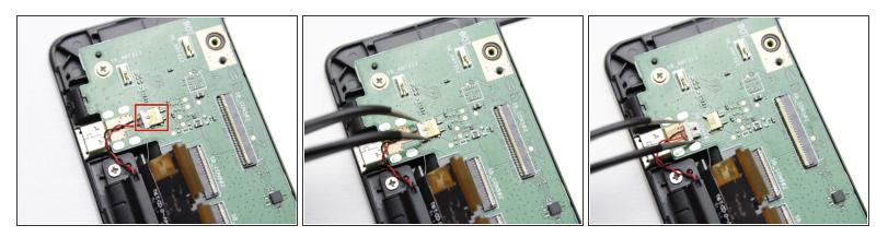
• Using the tweezers gently remove the connector from the yellow slot
