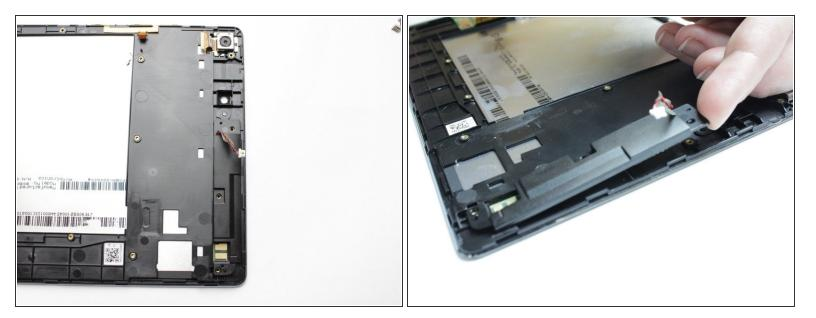
• Gently lift up the speaker to remove it from the device
