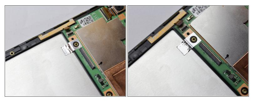
• Cut the warranty tape connecting the motherboard to the metal plate under the battery
