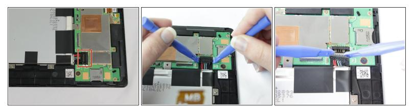
Remove the battery connector by prying it up away from the device using 2 plastic pry tools
