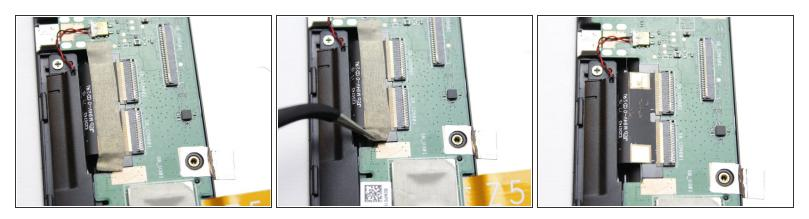
• Using the tweezers gently pull off the tape over the ribbon cable
