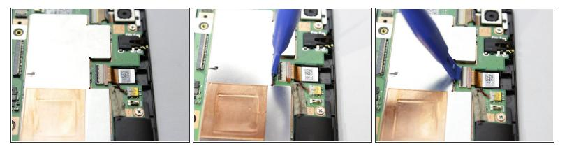
• Use a plastic opening tool to lift the black retaining flap on the ZIF Connector
