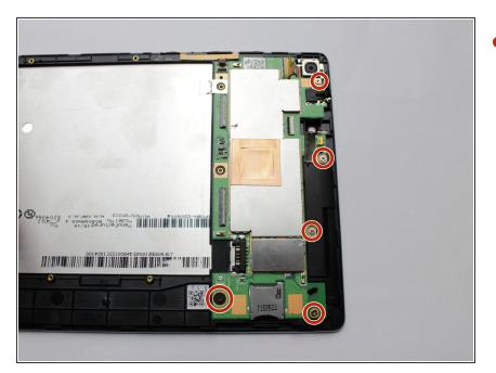
Using the #00 Phillips head screwdriver, remove the remaining 1.5mm screws in the motherboard
