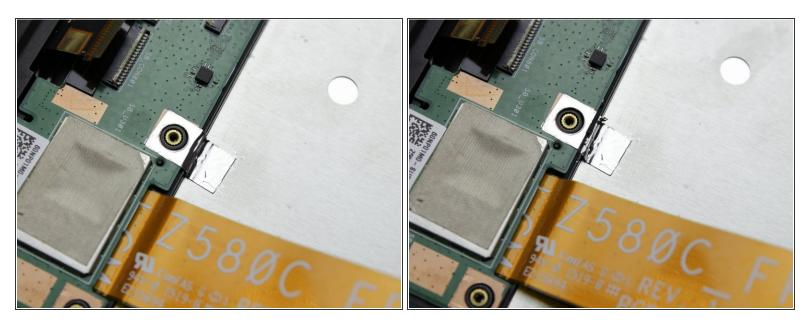
• Cut the warranty tape connecting the daughter board to the metal plate under the battery
