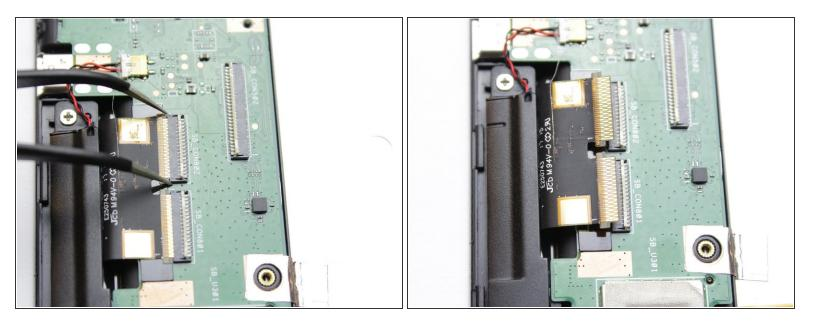
• Using the tweezers gently pull the ribbon cable out from from the connector.
