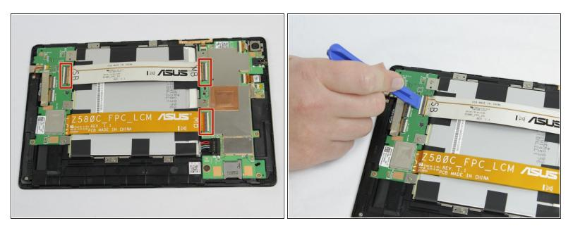
Remove the ribbon cables by lifting up the white retaining flap on the ZIF connectors, then pulling the ribbon cable away.
