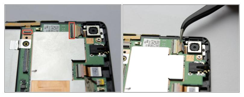
Using the plastic prying tool, lift the small retaining flap on the ZIF Connectors holding the ribbon cables to the motherboard
