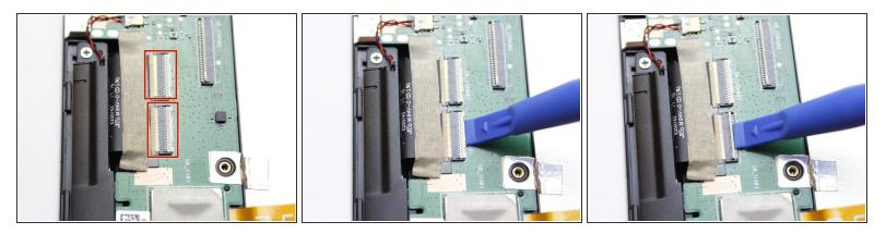
To remove the ribbon cables, lift up the white retaining flap on the ZIF Connectors with a plastic pry tool
