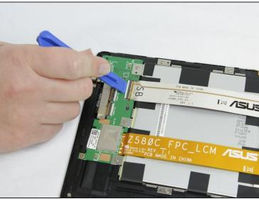
Remove the ribbon cables by lifting up the white retaining flap on the ZIF connectors, then pulling the ribbon cable away.
