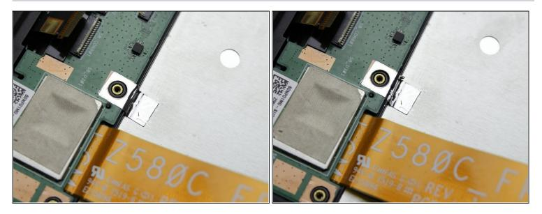
• Cut the warranty tape connecting the daughter board to the metal plate under the battery
