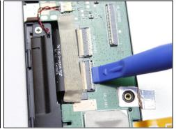
• To remove the ribbon cables, lift up the white retaining flap on the ZIF Connectors with a plastic pry tool
