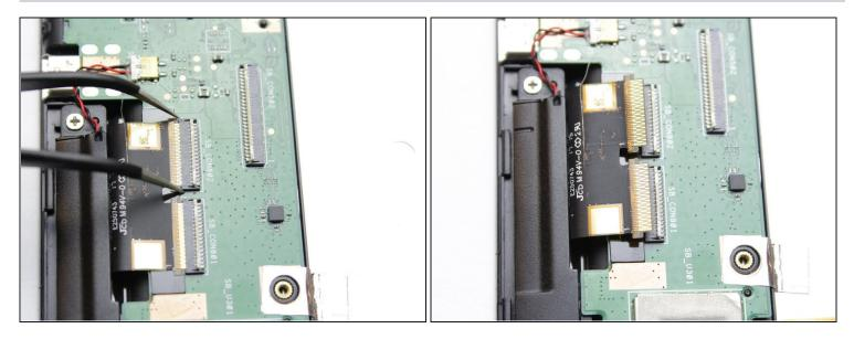
Using the tweezers gently pull the ribbon cable out from from the connector.
