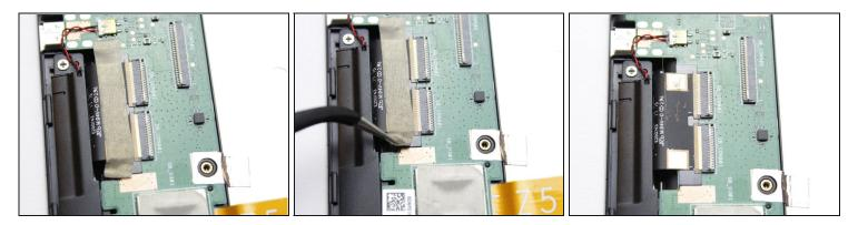
• Using the <u>tweezers</u> gently pull off the tape over the ribbon cable
