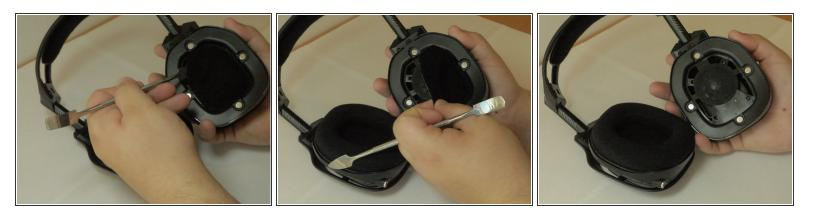
Remove the dust cover located on the speaker. Use the corner of the spudger to peel underneath the cover until you can lift it by hand. The cover is held onto the device with adhesive and should be removed slowly.
