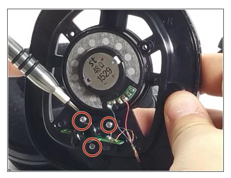
Remove the three screws in the photo with the J00 driver bit, and pull the headphone jack away from the assembly.
