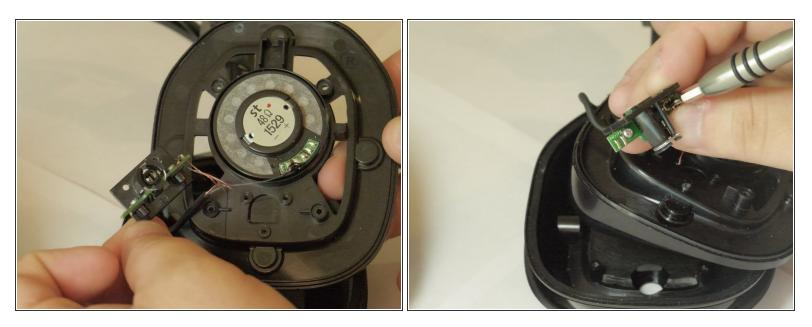
• Pull the motherboard off of the jack and replace it with a new one by re-soldering the wires.
