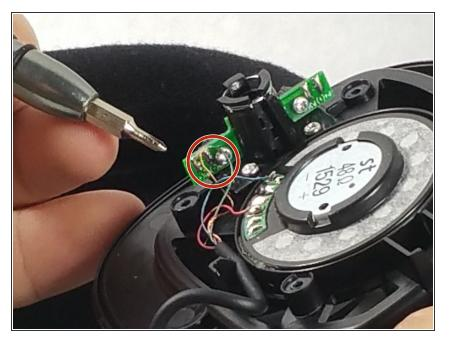
Un-solder the two wires circled, at this point the entire assembly can be removed from the speaker and the remainder of the device.
