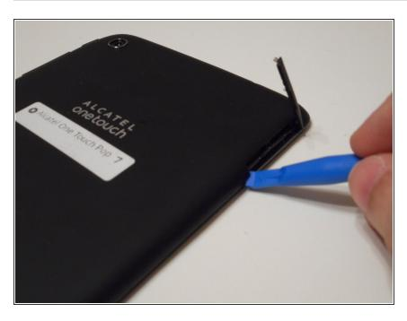
Begin working by using the plastic opening tool to remove the back cover of your Alcatel One Touch Pop 7. Opening the flap as shown in the picture will give you an easier start.
