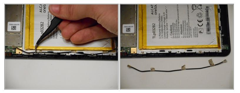
With each of the antenna ends disconnected, you can pull out the full antenna. There will be 3 pieces of tape wrapped around the antenna and stuck beneath the battery. They may be a bit difficult to remove but not impossible.
