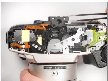
• Use the <u>tweezers</u> to gently remove the tripod socket, and replace it.
