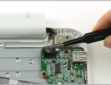
Use tweezers to lift the fabric cover and hinge connector away from the daughterboard.
