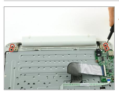
Use a Phillips #00 screwdriver to unscrew the four 6.4mm screws on the hinge mounts.
