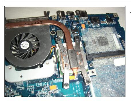
This is the CPU with the new alloy shim fitted.
