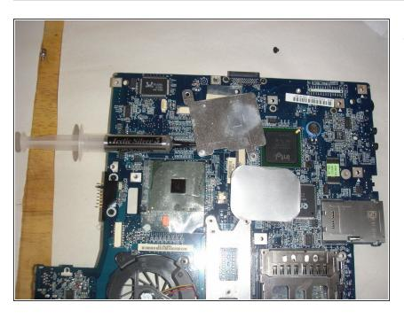
Thoroughly clean the chip with pure alcohol, then apply an even spread of good quality thermal paste(Arctic silver 5) will never let you down
