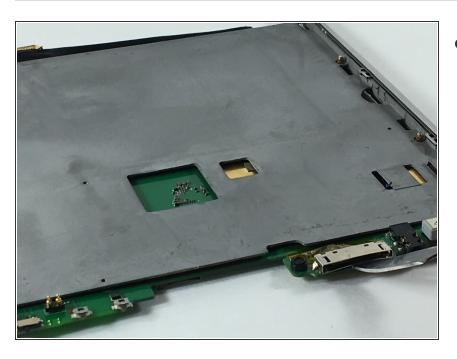
Use the metal spudger to pry off the charging port from the motherboard.
