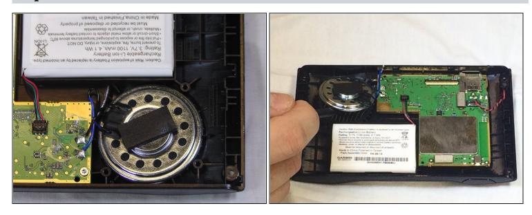
• Use your thin spudger to gently lift the speaker off of the sticky pad and away from the casing.
