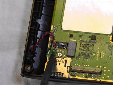
• Use your soldering iron to disconnect the wires from the motherboard. Disconnect the ground wire (the black one) and the positive wire (the red one).
