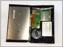
Use the plastic opening tool to pry open the device at the seam where the two halves meet, prying all along the sides and the top seams if need be.
