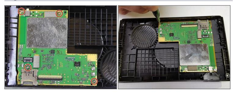
• Remove the four 4mm width by 5mm length T5 Torx screws using your screwdriver.
