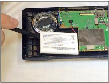
• Locate the battery and then use your spudger to gently lift the battery, which is held to the case using a sticky pad, and free it from its position.
