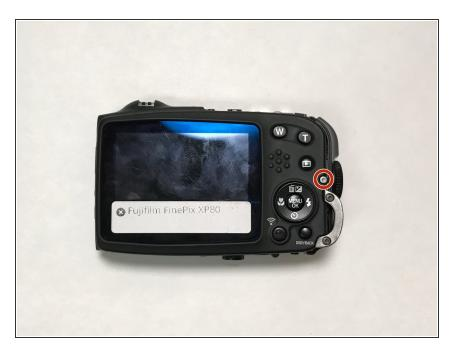
Using the H1.3 hex head bit, remove the screw on the back of the camera.
