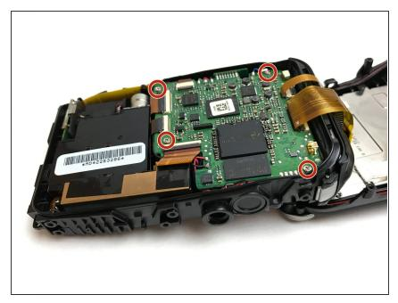
Using a PH000 Phillips bit, remove the four screws shown.
