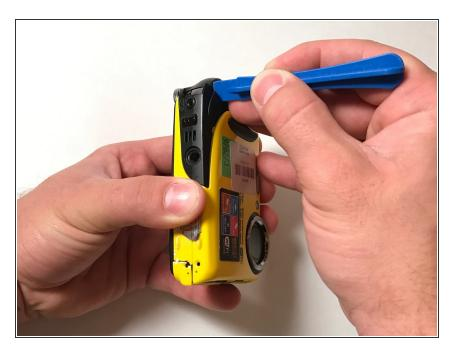
Continue using the opening tool on the bottom of the camera to gently pry the case apart.
