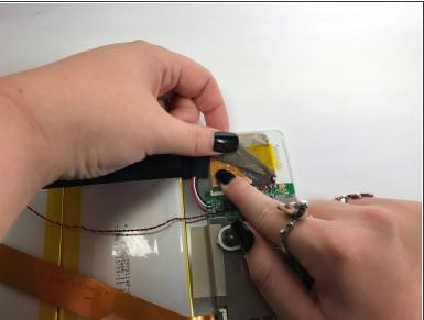
Using the plastic opening tool, remove the silver tape covering the display ZIF (zero insertion force)
