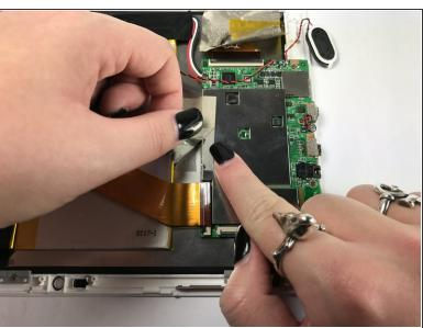
Using the plastic opening tool, remove the silver tape that secures the motherboard to the front panel.
