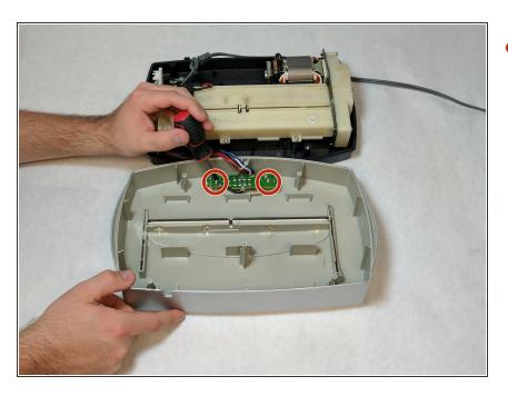
Unscrew both of the screws from the circuit board of the switch. Lift the circuit board away from the device.
