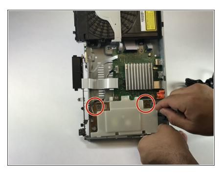
Remove both screws using the Phillips screw driver.
