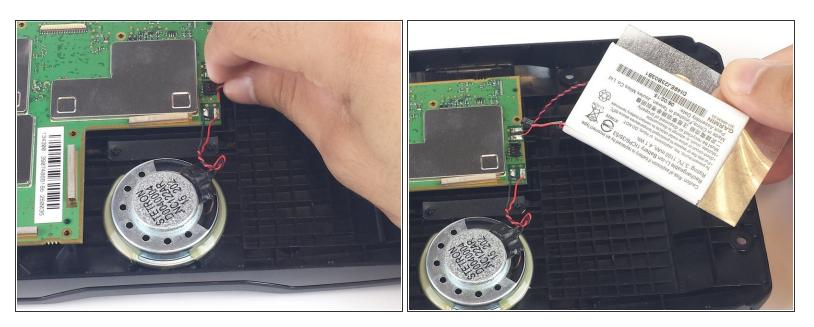
Grasp the wire near the mother board and gently lift to detach the battery.
