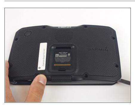
Place a nylon spudger in the seam between the front and back panel and carefully lift around the edge of the device.
