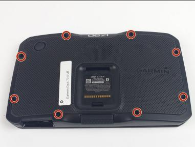
Turn the device screen down and using the screwdriver remove all eight screws from the back plate.
