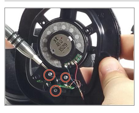
Remove the three screws in the photo with the J00 driver bit, and pull the headphone jack away from the assembly.
