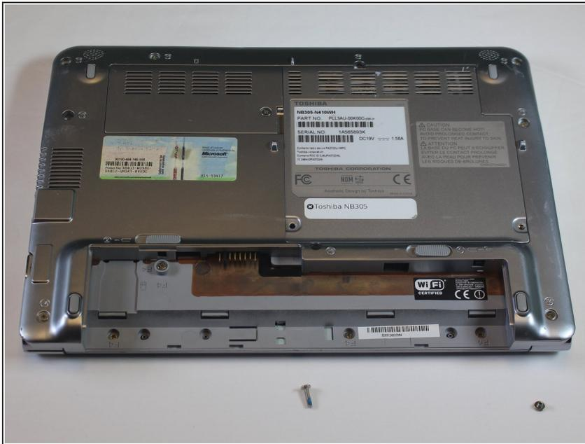
ⓘ Note that the screw on the left is longer than the screw on the right.
