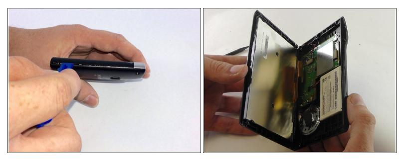
Use the plastic opening tool to pry open the device at the seam where the two halves meet, prying all along all sides if need be.
