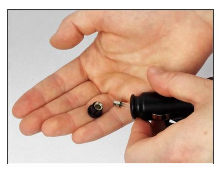
• Hold the charger at an angle so that the fuse comes out.
