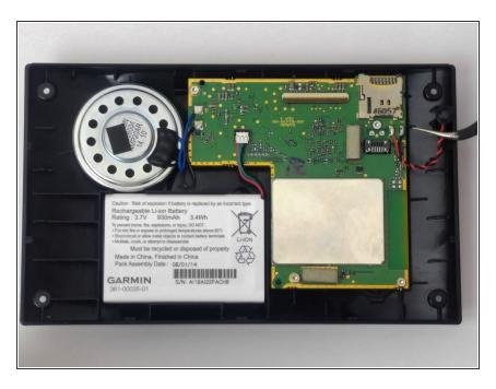
Using the angled tweezers, grab the microphone wires and gently pull to remove the microphone from the device.
