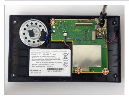
Using the T5 Torx Screwdriver, remove all 4 of the 4.0 mm screws from the motherboard.
