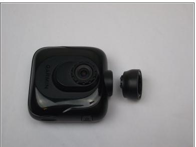
Remove the Dash Cam socket piece.
