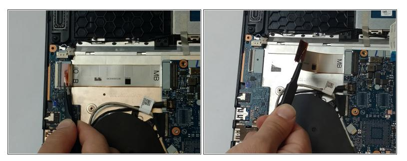
• Using the tweezers, carefully lift the black clip and remove the electrical ribbon.
