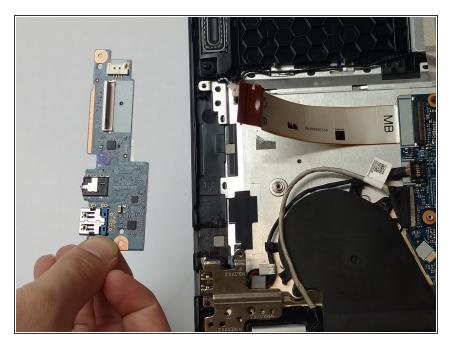
• The USB port is held in place by plastic pegs. Gently lift up to remove the USB port from the laptop.
