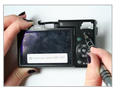
Using a Phillips #00 screwdriver, remove the 2.69 mm silver screw located beneath the plastic piece that was previously removed.
