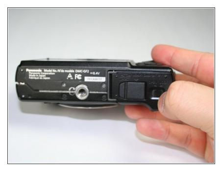
On the bottom of the camera, use your finger to push the lock button to the open position which will cause the hinged door to swing open.
